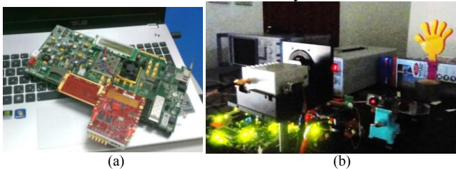
Fig. 12. The hardware platform that is used to build the prototype: (a) Xilinx ML605 FPGA board with .4DSP FMC126 high speed ADC and conventional laptop installed with Matlab. (b) APD C5658 mounted with optical lens.
