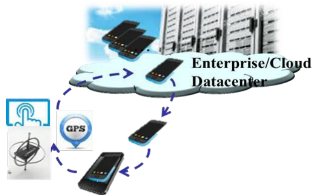
Figure 3 Virtual Mobile Infrastructure keeps apps and data in enterprise's datacenter and thus no data leakage risk
