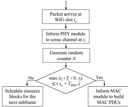
Fig. 11. A control flow chart that RSCH informs the MAC module to build MAC PDUs.
