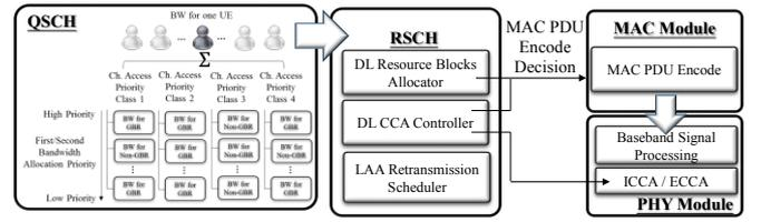
Fig. 9. The main functional components of RSCH and the communications between RSCH and MAC.
